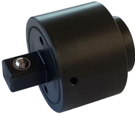
The DMB torque limiter is a factory torque set equipment, providing an over torque safety function without needing any maintenance during lifetime. In standard version it is designed with two connection for square drives in 3/8" and 1/2". As the DMB is a VMA developed and produced product the possibility for adaption on customer needs is very high. Special torque requirements as well as customized connections can be offered on request.
